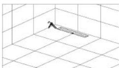
10. Fill silicone between floor drain and ceramic
