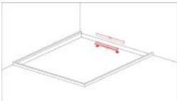
4. Put the shower drain in place and use spirit-level to ensure the horizontal surface around it.
